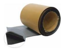
At first, remove masking paper slowly and evenly, and stick the tape bands at the mountpoint. When long bands are required, remove the paper successively to avoid tape corrugation. Press and smooth the stuck fragments out. At the end, remove the protective film, immediately before the next layers are stuck (eg. EPS, XPS or protective boards).
